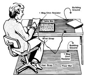
Figure 1-1. Static-safe Work Station
